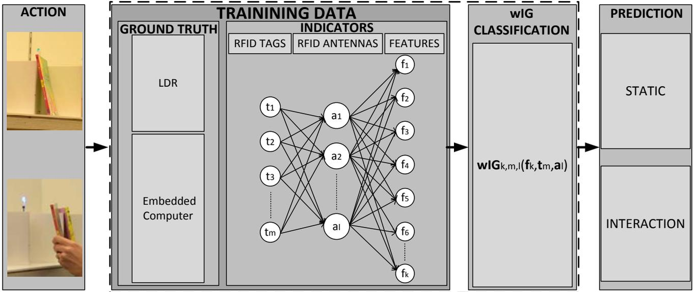
Fig. 2. Elements participating in the user-object interaction detection system.
