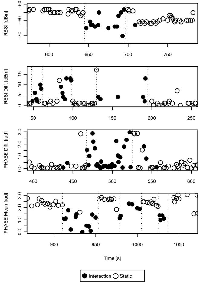
Fig. 1. RFID indicators like RSSI and Phase may describe object movement, which can be inferred as interaction with persons. Interaction and static samples in this figure are automatically determined by an LDR sensor.
